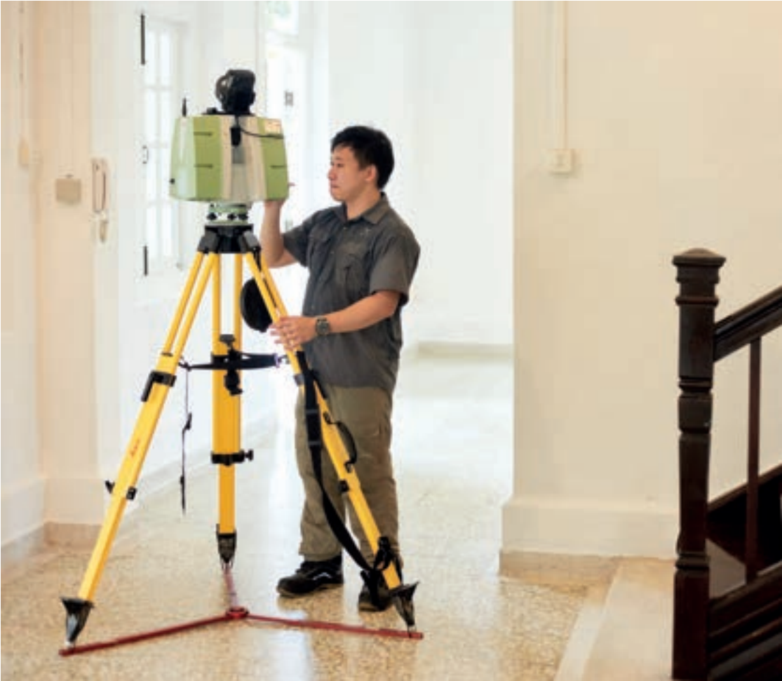
A 3D Terrestrial Laser Scanner in action, capturing a 3-dimensional image of this Black and White’s interior.
